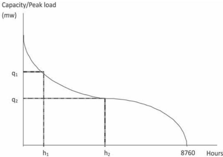
**Fig. 1: Load duration curve**
